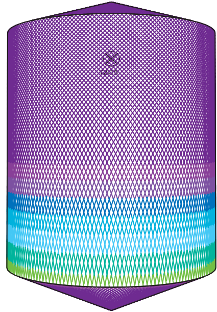
D8m H10m, Toftejorg MJ50, 4 x ø10 mm, 0 % Time = 23.3 min., Water consumption = 10868 l
