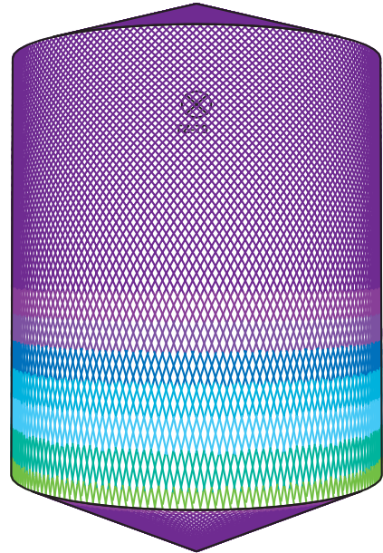
D8m H10m, Toftejorg TZ-79, 4 x \varnothing 10 mm, 0 % Time = 23.3 min., Water consumption = 10868 l
